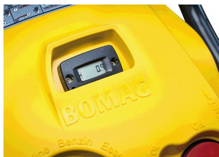
More transparency Hour counter/tachometer with a service indicator which can be reset
