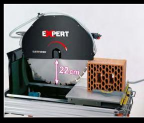
The cutting position with sliding carriage.
