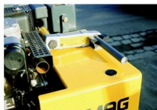
Simple and reliable to start Electric starter and hand starter
